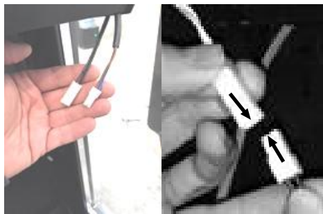
Fig. 7: Connect cable to LED-bar
